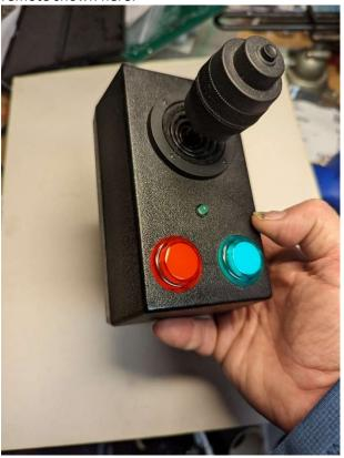
The "fire" button located at the top of the joystick is very convenient to use with gameplay. You can play with one hand, and don't have to remove your hand from the joystick control to send button commands.
