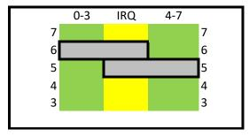
The output from the Cascade Interrupt Controller is sent to one of the native H8 interrupts. IRQ0-3 can be sent to a different H8 INT than IRQ 4-7. The example shows IRQ 0-3 to INT6 and IRQ 4-7 to INT5. Construct a 1x3 shorting jumper if you want all eight cascade channels to go to a single INTx.
