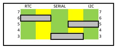
To use H8 INTerrupts, place a jumper over the desired INT line in one of the yellow columns and the matching pin in the source column. The example shows RTC->INT6, SERIAL->INT3, and I2C->INT5
